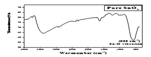
Fig.5 FTIR spectra of tin oxide nanoparticles
