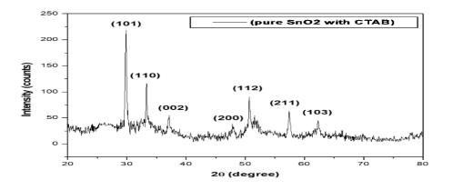
Fig 1. XRD pattern of pure SnO<sub>2</sub> nanoparticles
