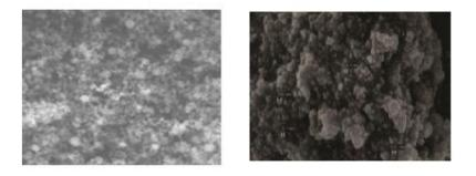
Fig.2.SEM images of the CuOand NiO nanoparticles
