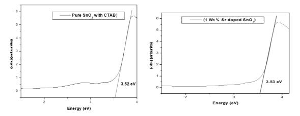
Fig 4(a) &(b) Tauc plot for pure and sr doped SnO<sub>2</sub> Nanoparticles
