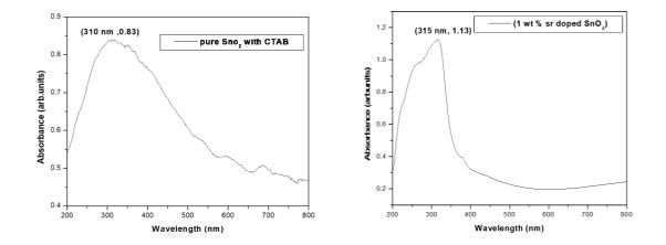
Fig.3 (a), (b)Optical absorbance spectra for pure and Sr doped SnO<sub>2</sub> tin oxide nanoparticles
