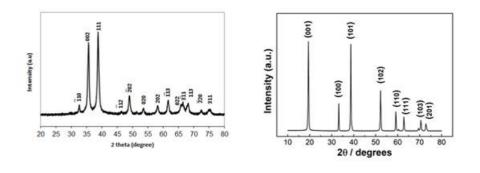
Fig.1. XRD patterns of CuO and NiO Nanoparticlescalcined at 550°C
