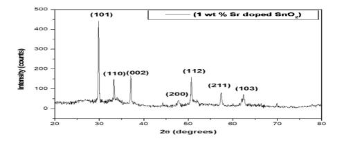
Fig.2. XRD pattern of 1 wt % Sr doped SnO<sub>2</sub> nanoparticles
