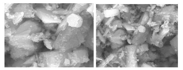
Fig. 6(a)(b) FESEM image of pure and Sr doped SnO<sub>2</sub> nanoparticles
