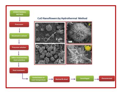
Fig.2. Schematic Illustration of Hydrothermal Synthesis of CuO Nanoflowers
