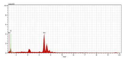
Fig.7 EDAX spectra of SnO<sub>2</sub> nanoparticles
